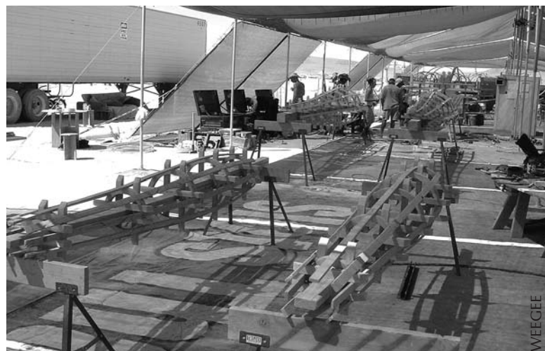
Wednesday afternoon, in the woodshop under where the man reposes. Department of Public Works is speed manufacturing a new man. Legs, arms and torso are well along to completion. Only a face piece with some charred wood and melted neon tubing is being reused.
